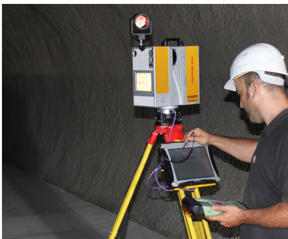
TMS Tunnelscan application using Amberg Profiler 5033
