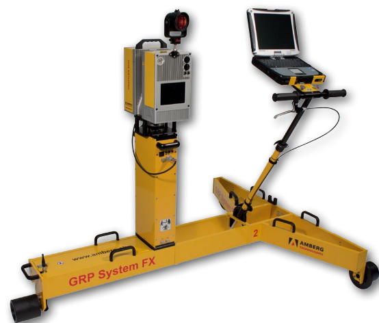
GRP 5000 System with Amberg Profiler 5033
